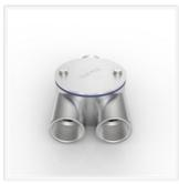
Electrix® Metric Conduit Three Way Boxes, in 316C16F stainless steel with a 316L - V4A - 1.4404 stainless steel lid, can be used to change direction during an installation and to provide an additional outlet for conduit runs, whilst the removable lid provides access for inspection and installation purposes.
